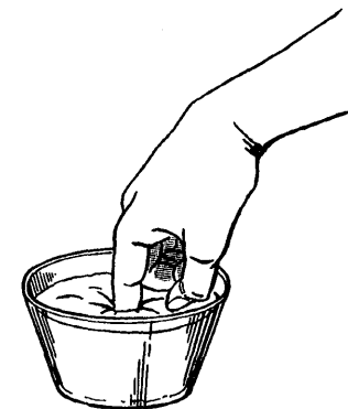
Figure 6.3 A finger immersed in mercury. The pressure deep in the liquid is much greater than that at the surface but only the discontinuity is experienced.
